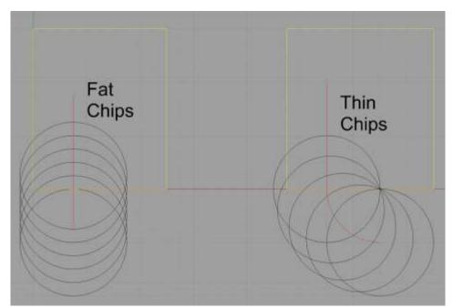
Not the chip shape to the right of the feed line (the red line is the path the cutter follows): thin chips on exit are better!
